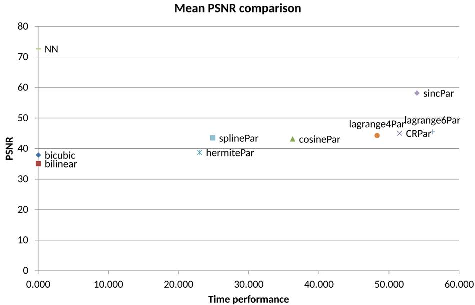
Fig. 3. Comparison of mean peak signal-to-noise ratio method (PSNR) estimator with mean time elapsed during calculations for tested interpolation methods.
