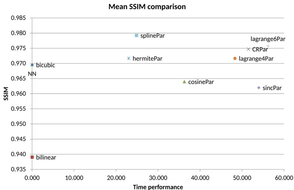
Fig. 4. Comparison of mean structural similarity (SSIM) estimator with mean time elapsed during calculations for tested interpolation methods.
