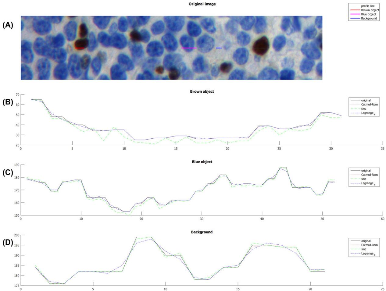
**Fig. 6.** Comparison of interpolation performance. Comparison is performed for brown (B) and blue (C) object and background (D) fragment, marked by colour segments on the white profile line (A). Original values (black line) are compared with values after interpolation performed with recommended functions: Catmull–Rom (red dotted line), sinc (green dashed line) and Lagrange (blue dash-dot line). For clarity only blue channel (of RGB) is showed. Interpolation scale: 0.9.
