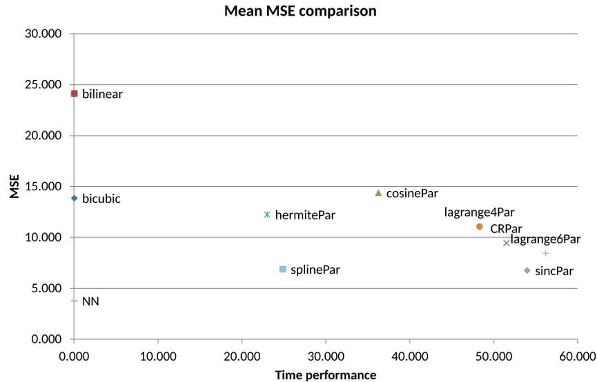
Fig. 2. Comparison of mean mean squared error (MSE) estimator with mean time elapsed during calculations for tested interpolation methods.
